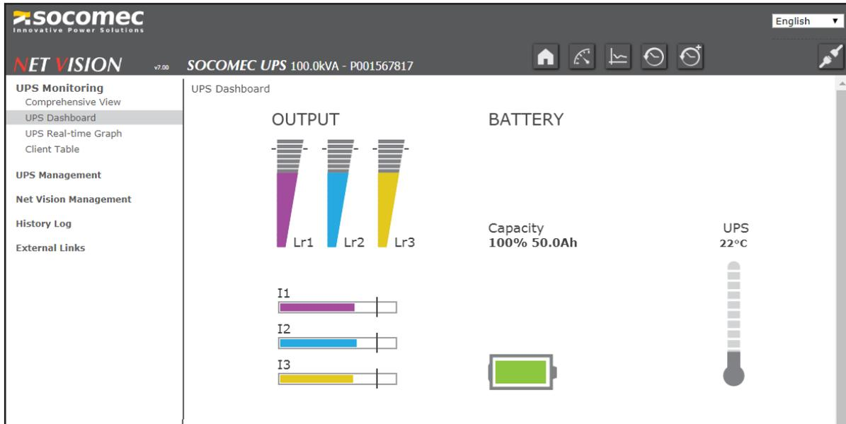
During battery discharging, remaining backup time is displayed
