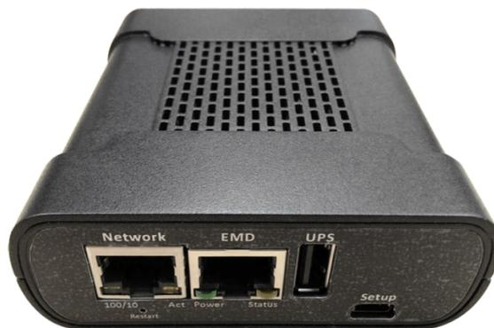
The Network RJ45 connector is used for Ethernet network connection.
