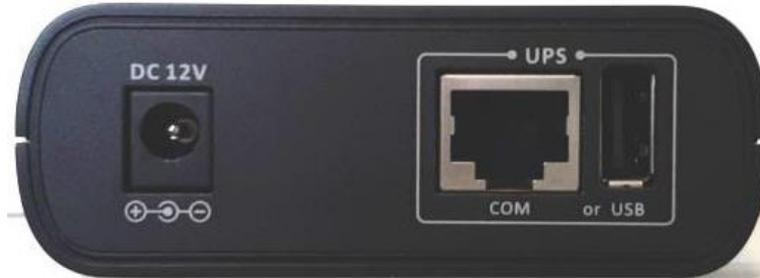
The serial link to UPS is located on the back of the box. The serial cable included in the package has to be connected to 'COM' RJ45 connector and to the UPS RS232 DB9 serial port.
